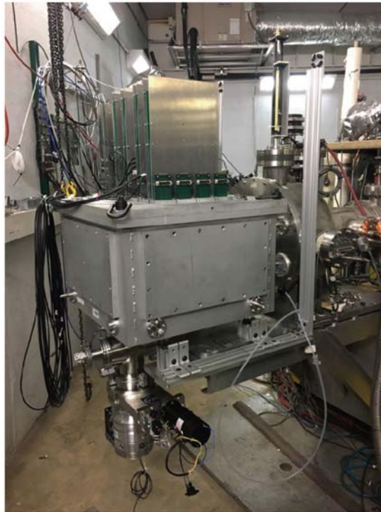
FIG. 2. A photo of TexAT full setup for an experiment with RIB beam. AsAd motherboards are placed on top of the TexAT chamber.
